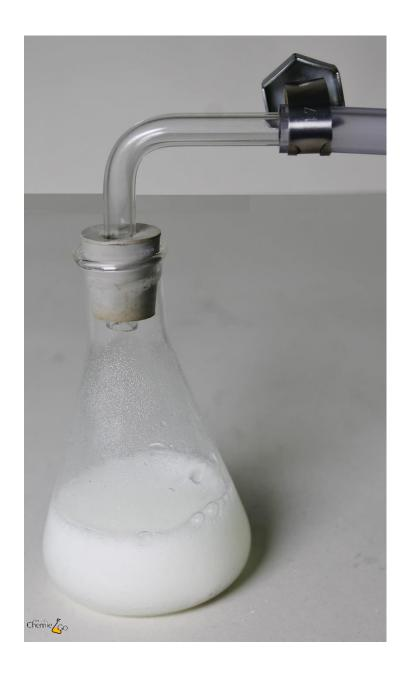
The Erlenmeyer flask is also used for reactions with gas evolution. The gas produced can be discharged via a glass tube (gas discharge tube).
