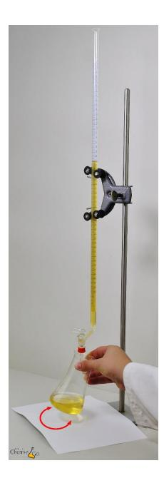
During a titration, the solution in the Erlenmeyer flask is swirled so that the solutions mix well. The conical shape prevents the solution from splashing out.
