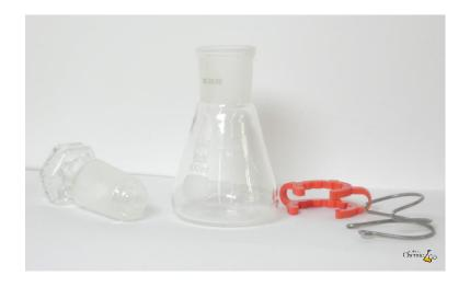
The stopper can be secured with a clip from metal or plastic.
